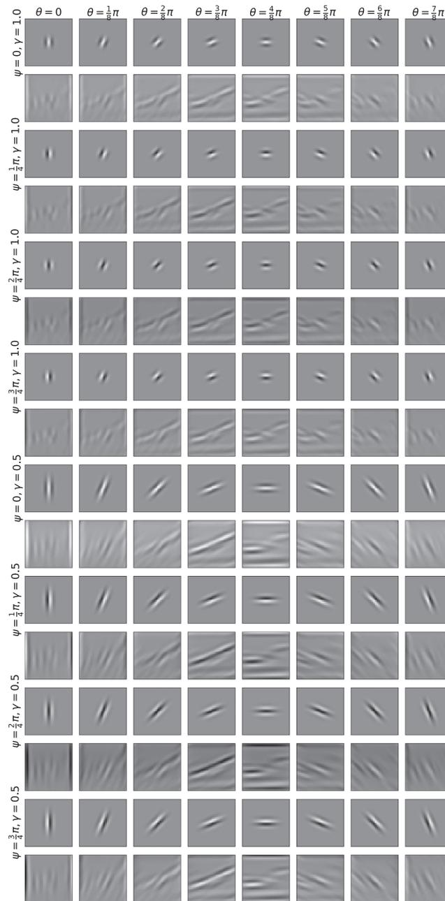
Fig. C.11. Illustrative set of Gabor filters used in the first convolutional layer of the network with  $\lambda = 5$  and  $b = 1.4$ . Orientation ( $\theta$ ) varies from 0 to  $\frac{7}{8}\pi$  across each row, while down each column  $\psi$  varies from 0 to  $\frac{3}{4}\pi$  and  $\gamma$  varies from 1 to 0.5. The Gabor kernels are displayed on odd rows while the results of their convolution with an example image from the training set (Fig. 2) are shown on even rows.
